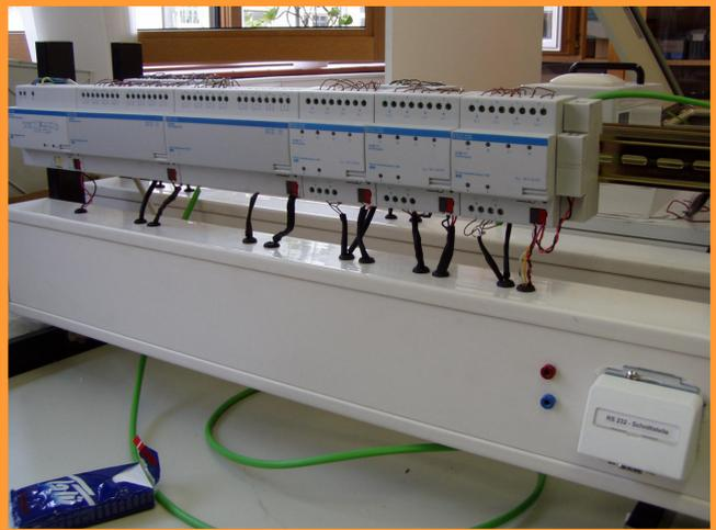
Within the scope of a diploma thesis the functionalities of Siemens S7-300-, S7-200- and Logo-systems are analyzed for the tasks of building control systems. The compatibility of big and small SPS-automation-systems with EIB-installations using gateways is analyzed too.
